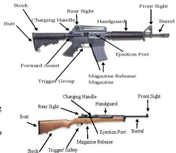
(Figure 2-6) Rifle/Carbine Position of parts may vary depending upon the make and model of the weapon.
