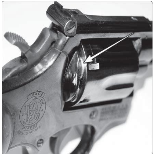
(Figure 6-2) Cylinder placement with partial load
